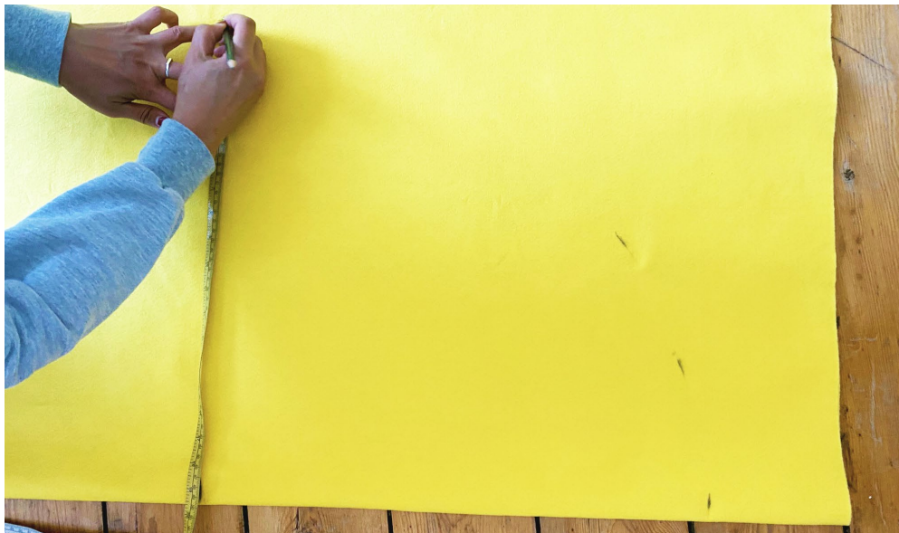
Fold your seating circle fabric in half. Mark out a half circle - it should have a radius of 500mm.
