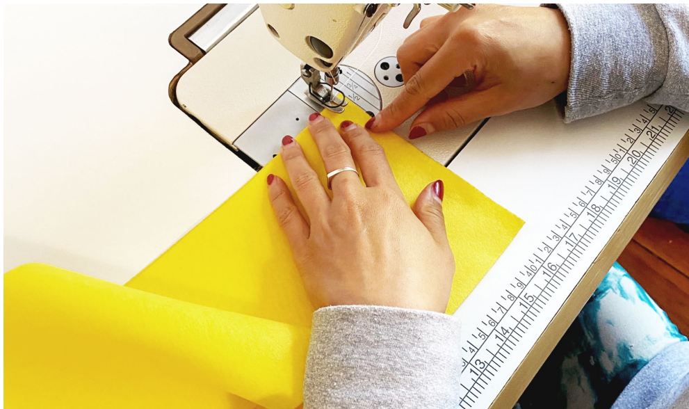
Sew along the 1cm overlap, using the small cuts as a guide
